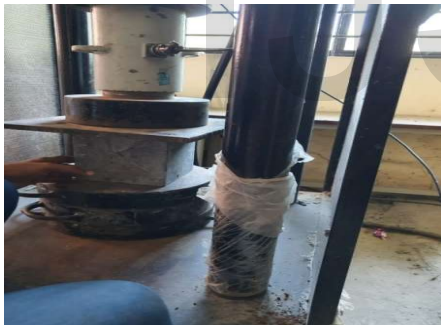
Figure 6 : Cube placed in CTM for loading
